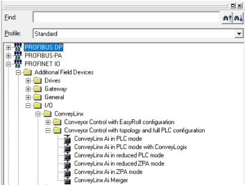
Drag and drop the **ConveyLinx Ai in PLC mode** into the network and assign the Conveylinx object to the controller.
