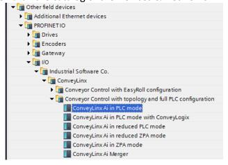
Drag and drop the ConveyLinx Ai in PLC mode into the network. Assign the Conveylinx object to the controller.
