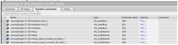
The .....~virtual\_input\_module\_64\_byte\_1 must be linked to the "Hardware identifier Input" and the ~virtual\_output\_module\_64\_byte\_1 must be linked to the "Hardware identifier Output". The linking can be done by selecting the tag and dragging it to the input of the function block you want to link this module to. It can also be done by just typing the number which is in the hardware identifier column at the input of the function block.
