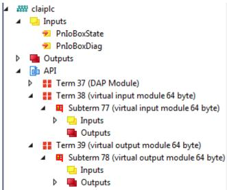
Make sure that the checkbox **Swap LOBYTE and HIBYTE** is checked! This can be found under the controller -> API -> Term (Virtual input module 64 byte) -> Inputs -> Inputs. Double click on the Inputs and go to the tab "Flags". Check the checkbox **Swap LOBYTE and HIBYTE.** Do this also for the outputs!
