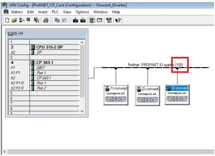
In this example the CPLADDR is **W#16#100**. Use Mode **B#16#0**. The LEN parameter depends on the number of Modules needs to be read out. 1 diverter needs 64 bytes, in this example 3 diverters are configured so 3x64 = 192 bytes. The Data area for the data of the diverters is put at the RECV IO from the function block. This data area needs to be linked to the Flowsort Function block.
