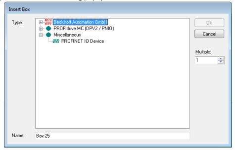
Select the PROFINET IO Device under miscellaneous and click OK. Now select the folder where the unpacked GSDML file is located. Select the .XML file and click Open. The following popup will be shown. Select the **ConveyLinx Ai in PLC mode** and click OK.
