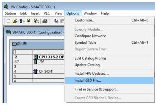
In the following popup select the path of where the GSDML file from the diverter is downloaded and install the GSDML file. When the installation was done correctly, the device is now available in the hardware catalog.
