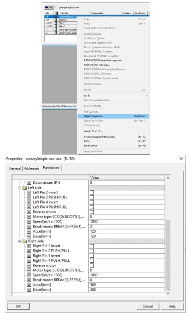
The speeds and ramps (Accel/Decel) are send in the program so it is not necessary to set the speed in the configuration of the controller. The values used here are only used after a communication failure as "initial values".
