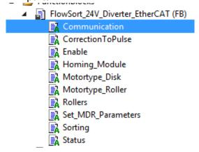
The **MotorType\_Disk** part scales the speed values from the disk from 0 - 100% to pulses to send to the controller
