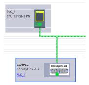
Now the system integrator can give the module an ProfiNET name and IP-adress.
