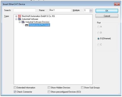
Select the MotionLinx-AI PLCmode and click OK. Now the MotionLinx-Ai Controller is added to the project. In the Solution Explorer the MotionLinx-Ai Controller is available with all the data.
