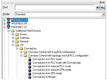
Drag and drop the **ConveyLinx Ai in PLC mode** into the network and assign the Conveylinx object to the controller.
