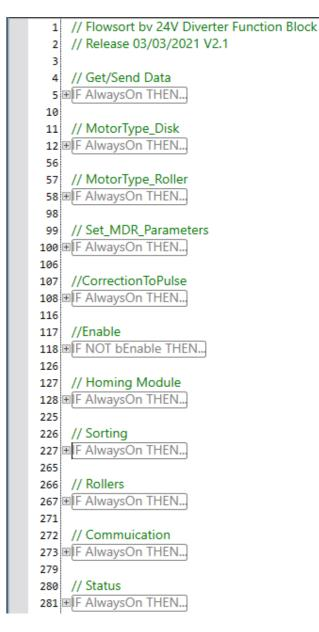
The **Get/Send Data** parts reads out the data from the Ethernet/IP Device and sends the data to the Ethernet/IP device with the given Hardware data and convert the data to values . The **MotorType\_Disk** part scales the speed values from the disk from 0 - 100% to pulses to send to the controller
