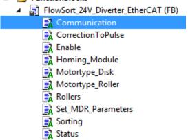
The **MotorType\_Disk** part scales the speed values from the disk from 0 - 100% to pulses to send to the controller
