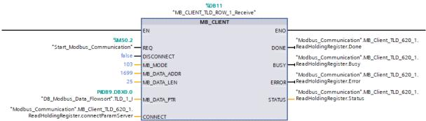
For receiving modbus data, function block **MB\_CLIENT** is used. To get the right data from the conveylinx module the inputs:
