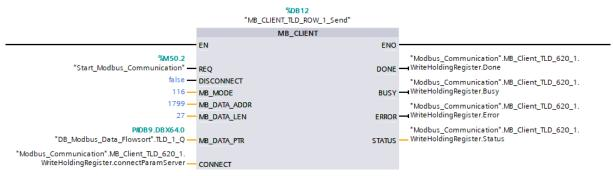
For sending modbus data, function block **MB\_CLIENT** is used. To send the data to the right place in the conveylinx module the inputs:
