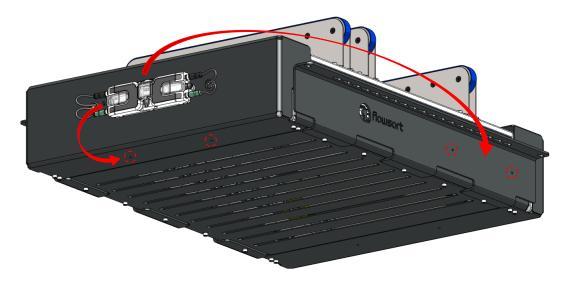
Control card can be relocated to the bottom of the covers or to the flanges:
